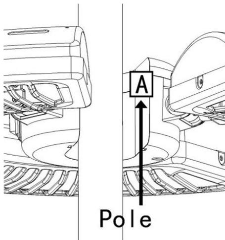
**Step 2:** Slip the Mounting Part **B** and fit it to the Mounting Part **A** from the bottom up.
