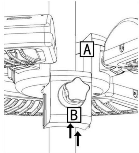
**Step 3:** Turn the Fixation Screw until the Mounting Part **A** is fixed on the pole
