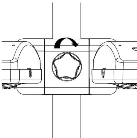
**Step 4: The machine can use 3 swing angles.**
