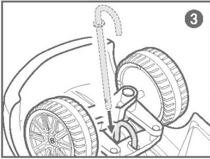
Install the steering wheel connection rod as shown.
