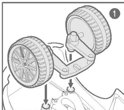
Turn over the semi-assembled main body and insert the front wheels into the designated location on the underside of the car
