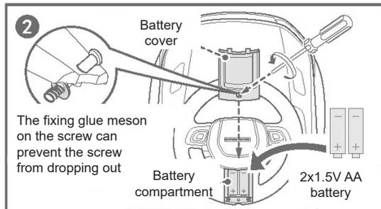
Open the steering wheel battery compartment and insert 2 x AA batteries taking care to ensure that each battery is inserted correctly. Replace the battery cover and secure with the screw provided.
