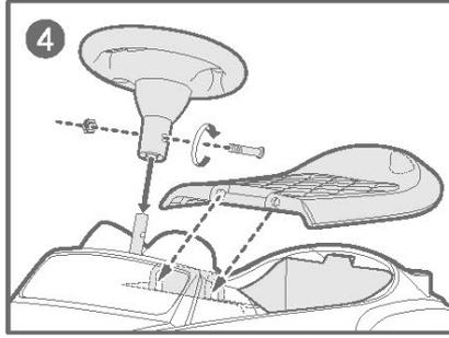
Insert the steering wheel into the top of the steering wheel connection rod and secure with the screws and screw caps. Install the seat as shown onto the main body.
