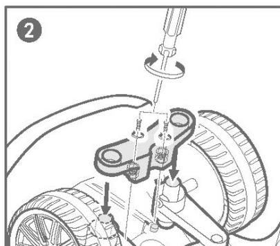
Insert the "I"-shaped frame into the designated location on the front wheel according to the direction of the arrows. Secure with screws provided.
