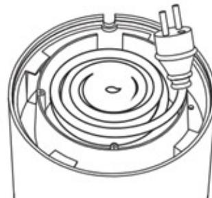
Step 2: Take the power cord out of the plastic box and let the power cord through the hole in the plastic box.
