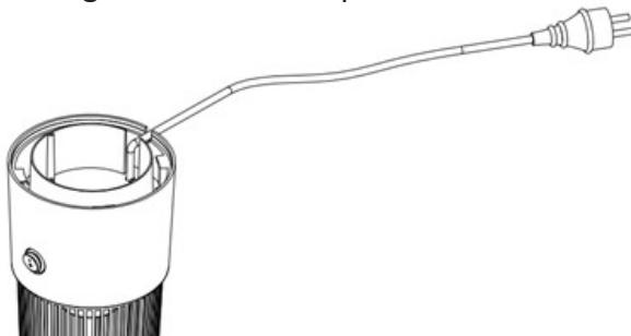
Step 3: Cover it with the plastic cover and tighten it clockwise.
