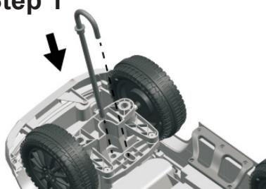
**How to assemble the J-shaped stick** - Install the J-shaped stick at the assigned location as picture.
