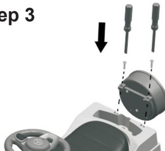
**How to assemble the spare tire**
